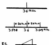
If a carrier Is modulated by a band of frequencies, such as speech, then both upper and lower sidebands will be produced.
