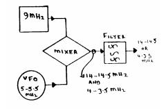
This example would permit operation on Metres(3.5-3.6MHz) or 20 Metres(i4-14.35MHz) bands.
