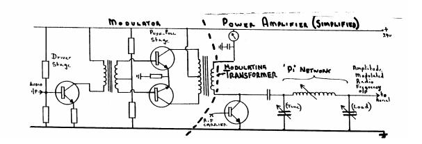
It is very Important to ensure that over-modulation never occurs. This would produce many harmonics and spurious sidebands. These extra side bands will result in a very 'wide' signal taking up far too much of the frequency band. It is best to aim for a maximum of 90%. This will leave a safety margin of 10%
