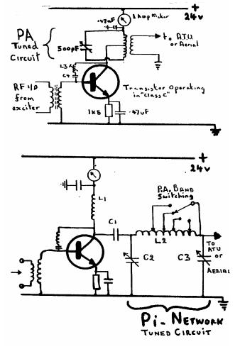
The Pi circuit has the additional advantage of much higher harmonic rejection. The second harmonic rejection is four <u>times</u> better a conventional parallel tuned circuit.
