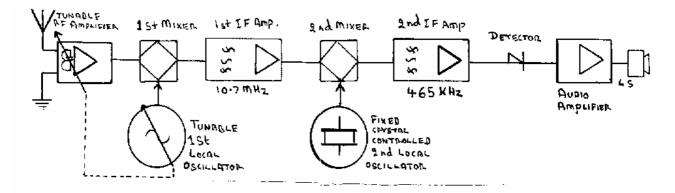
The signal is amplified by the tuneable RF amplifier and then mixed with the first local oscillator to produce the first IF 10.7 MHz. The real purpose of the 10.7 MHz IF amplifier is to prevent "image frequency" problems. It is then converted to ~65 kHz by the second mixer. As both IFs are, of course, fixed frequencies the second LO is also fixed. The second LO will be either 10.7 + 0.465 or 10.7 - 0.465 MHz and is a crystal controlled oscillator.
