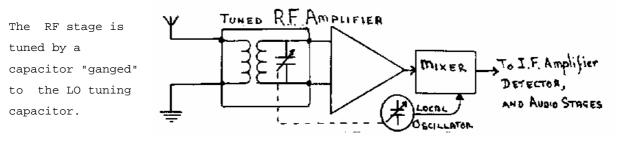
In a superhet there are no feedback problems as a result of using a ganged capacitor as the sections are now operating at different frequencies.
