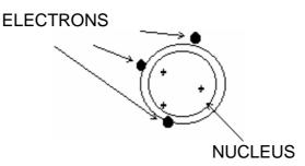
Each atom comprises a nucleus (in the centre) and one or more orbiting electrons. The electrons each have one negative charge.
