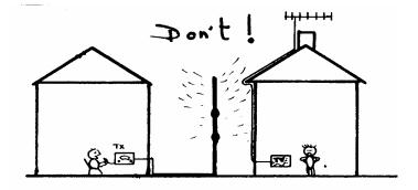
The transmitting aerial should be sited away from any TV's or .Hi-Fi's and their aerials or cables. Efforts should be made to minimize the coupling between the transmitting s>'stem and the TV coax by not having the two running parallel. For example, it would be unwise to Install a vertical amateur aerial anywhere near where the TV coax runs up the wall to the roof.
