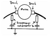
It was soon recognized that such interference was antisocial. However, it was quite easily avoided - each motor was manufactured with a suppressor" fitted. This damped the spark and greatly reduced its annoying radiation. The circuit although simple, was generally effective. Add-on suppressors then became available to fit to earlier un-suppressed motors.
