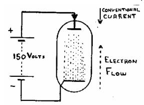
Thus, with the .High Tension battery connected as shown there will be a strong stream of electrons flowing, across the vacuum, from Cathode to Anode. If, however, the battery were turned round, the then negative Anode would repel the negative electrons and the flow would cease.
