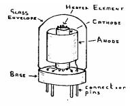
By heating the metal (called the cathode) the electrons become very agitated and many of the electrons escape from its surface.
