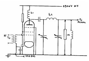
The "+300V" is connected to the anode via inductance L1 which will pass the anode current but block the Radio Frequency.
