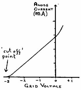
If the grid is not connected to anything, it won't have any effect. However, a small negative voltage on the grid will make a difference. The negative grid will repel some of the negative electrons and therefore cut down their flow from Cathode to Anode. The actual effect on the flow depends on the size of the negative voltage (grid bias) as can be seer, in the graph on the left. It shows the relationship between the negative grid bias and the Anode current.
