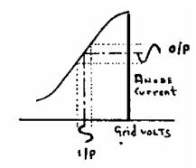
This Shows a valve biased to operate in the middle of the straight section of the anode current/grid voltage graph.
