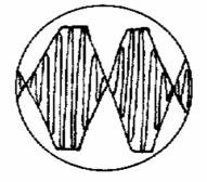
Could be the result of *over driving* the Power Amplifier stage of the transmitter. There is intermodulation.
