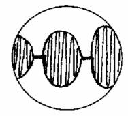
Perhaps due to incorrect bias of the power Amplifier stage of the transmitter. There is intermodulation.
