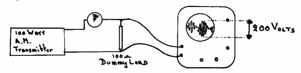
The 100 watt carrier is then fully amplitude modulated.(100%) by a sine wave audio tone. The resultant RF output is displayed on the oscilloscope. The radio frequency is very high compared with the audio frequency and the individual RF cycles may merge into each other on the screen and just appear as a green "modulation envelope".
