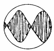
This is the "good" waveform. The peaks are correctly rounded and the crossover is sharp and straight. No intermodulation Indicates a fault.
