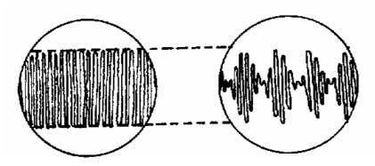
The waveform on the left is the display of the RF output of a SSB transmitter that has a single tone injected at the microphone input. As mentioned before, a single tone input will result in a <u>single</u> Radio Frequency output.
