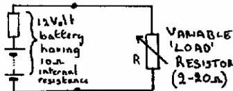
CALCULATION OF POWER IN LOAD RESISTOR
