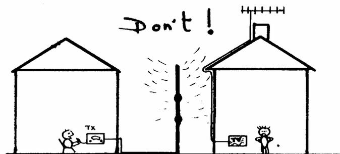
The transmitting aerial should be sited away from any TV's or Hi-Fi's and their aeriels or cables. Efforts should be made to minimize the coupling between the transmitting system and the TV coax by not having the two running parallel. For example, it would be unwise to install a vertical amateur aerial anywhere near where the TV coax runs up the wall to the roof.
