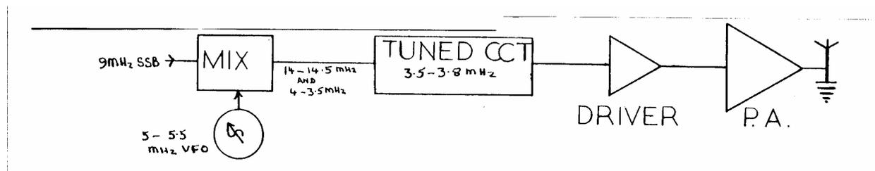
This transmitter uses the 9MHz SSB generator, at the top of the page, mixed with the output from a 5.0-5.5 MHz VFO.
