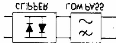
In order to avoid excessive bandwidth, due to these harmonics, the limiter should always be followed by a low-pass filter.
