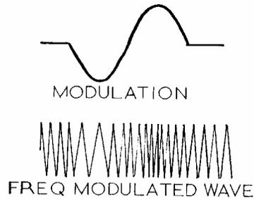
However, the Amateur License states that the bandwidth of an transmission must be no more than the 6 kHz permitted on AM. It is known Narrow Band Frequency Modulation (NBFM).
