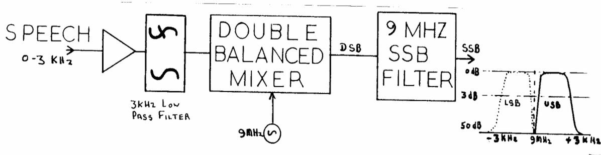
Speech, from the microphone, is amplified and connected via a low pass filter to one input of the double balanced mixer. The carrier, in this case 9 MHz, is connected to the other input.
