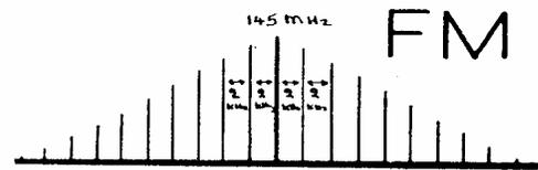
In theory there will be an infinite number of side frequencies at 2 kHz intervals. In practice, most of the energy is in the frequencies near to the centre. In fact, side frequencies remote from the carrier are very weak and can usually be ignored.
