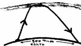
This is the lowest ionised layer that can usefully be used for ionospheric propagation. The E layer, which will quite happily refract (bend) radio waves during daylight hours, virtually disappears at night. being relatively low, the E layer does not normally result in vast distances of communication. The radio signals are refracted back to earth at distances of hundreds rather than thousands of miles away.
