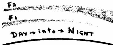
During daylight hours the F layer splits into two. The lower part (150-200 kms) disappears at night and the F2 layer approximately doubles its width. This upper (F2) layer is the most important ionised region for long distant communication using "sky waves".
