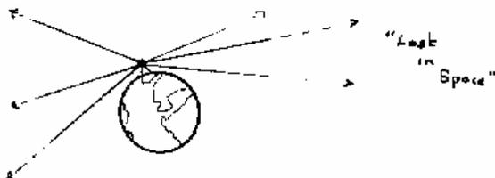
If the world had absolutely nothing around it the radio waves would carry on in straight lines and disappear into space... lost for ever.
