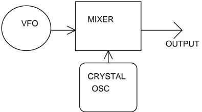
By using a variable frequency oscillator and a crystal oscillator feeding a mixer any frequency can be obtained. For example if a VFO in the range 5 - 5.5 MHz is used in conjunction with a 2.0 MHz crystal to give a mixer output of 7.0 - 7.5 MHz.. If a 23 MHz crystal is used there will be an output in the range 28 to 28.5 MHz.
