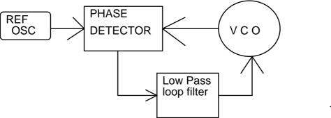
The simple phase lock loop circuit enables a Voltage Controlled Oscillator to be <u>exactly</u> locked to the frequency of the crystal controlled *reference oscillator*.
