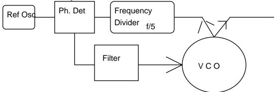
Remember that the *phase detector* will send an tuning voltage to the VCO to adjust both the frequencies fed to it to be the same.
