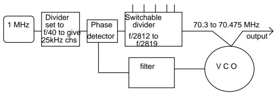
This shows how a *Phase Lock Loop system* can be used to generate frequencies at the required channel spacing for any Amateur Band. The example taken is 25 kHz channel spacing in a section of the 70 MHz Band. To adopt 12.5 kHz spacing , as suggested by the band plan, the fixed divider would have to be set to *divide by 80*, instead of 40.
