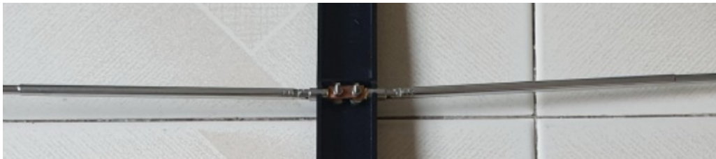
Telescopic antenna as Yagi elements
