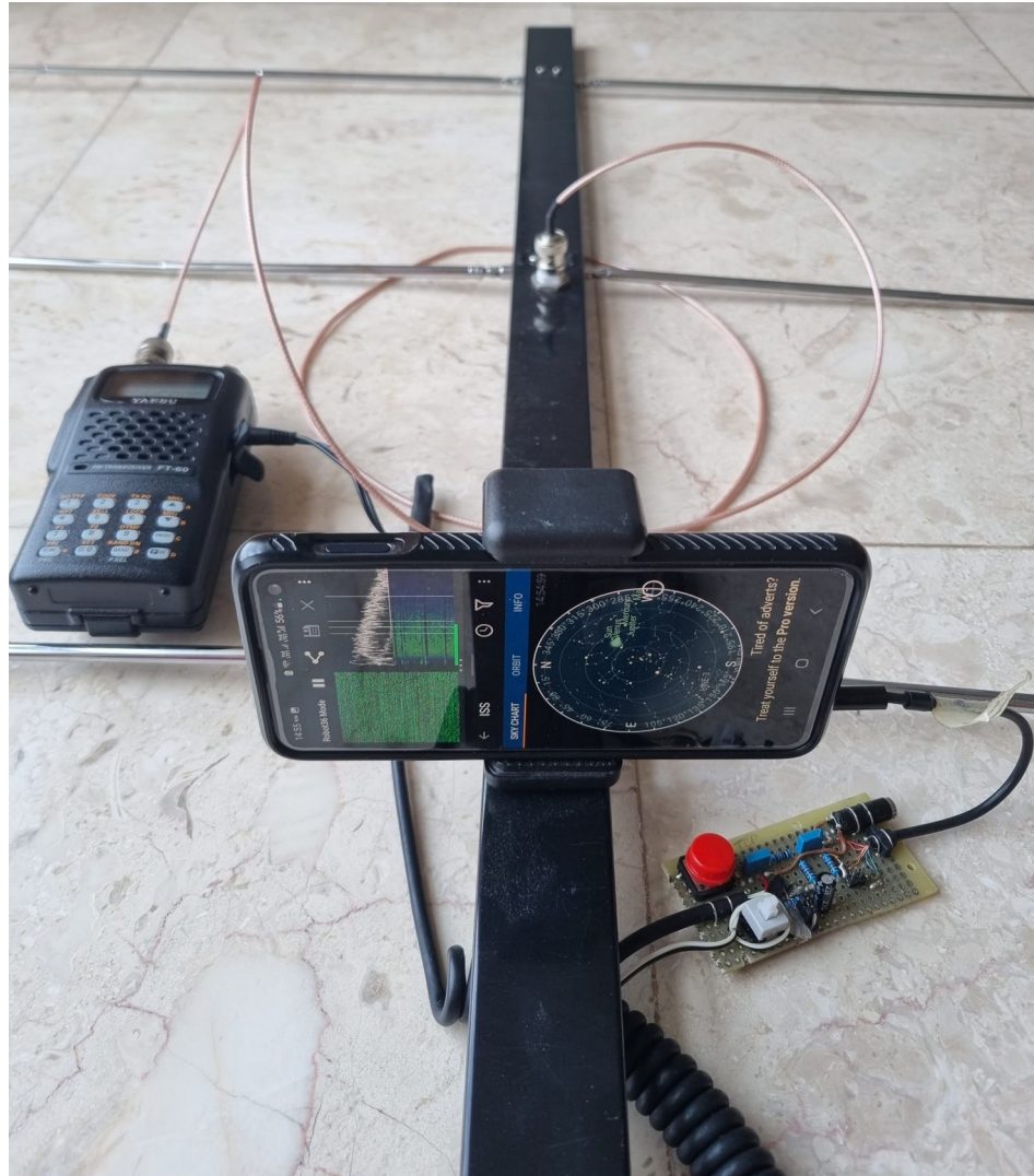
Yagi antenna with phone holder
